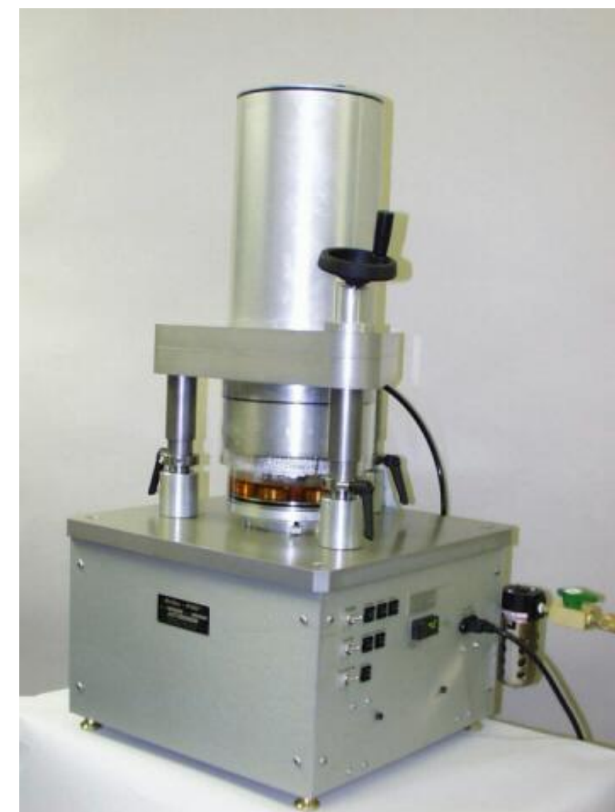
Figure 1. The AMTI Ortho-Pod machine is a six-station pin-on-plate type wear testing machine. The machine has three independently controlled variables, which are the plate rotary motion, the pins rotary motion and the normal load on the pins.
